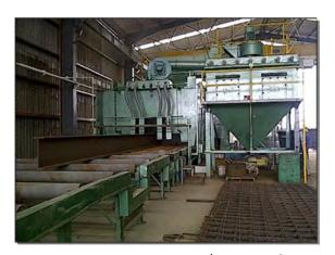
AUTO-BLAST MACHINE C/W INFEED & OUTFEED CONVEYOR
