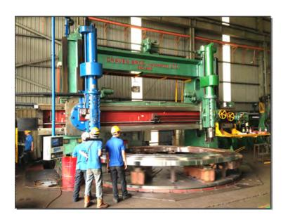
CNC- 18 FT CRAVEN VERTICAL LATHE TURNING & BORING MACHINE
