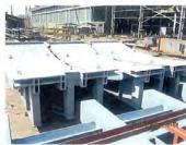
Settler Flash Furnace: Bottom Saddle (109.380 kg)
