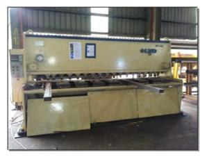
LVD SHEARING MACHINE 20mm x 3.0m
