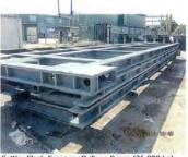
Settler Flash Furnace: Grillage Beam (26.800 kg)
