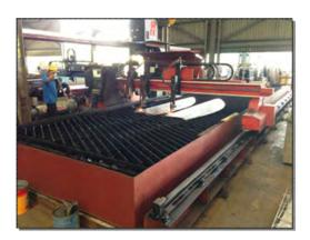
FUSION CNC PLATE OXY AND PLASMA CUTTING MACHINE
