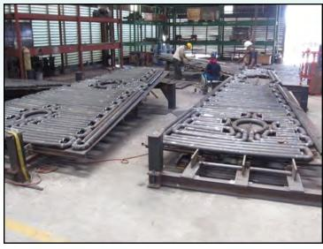
**Cooling Water Piping Circuits**
